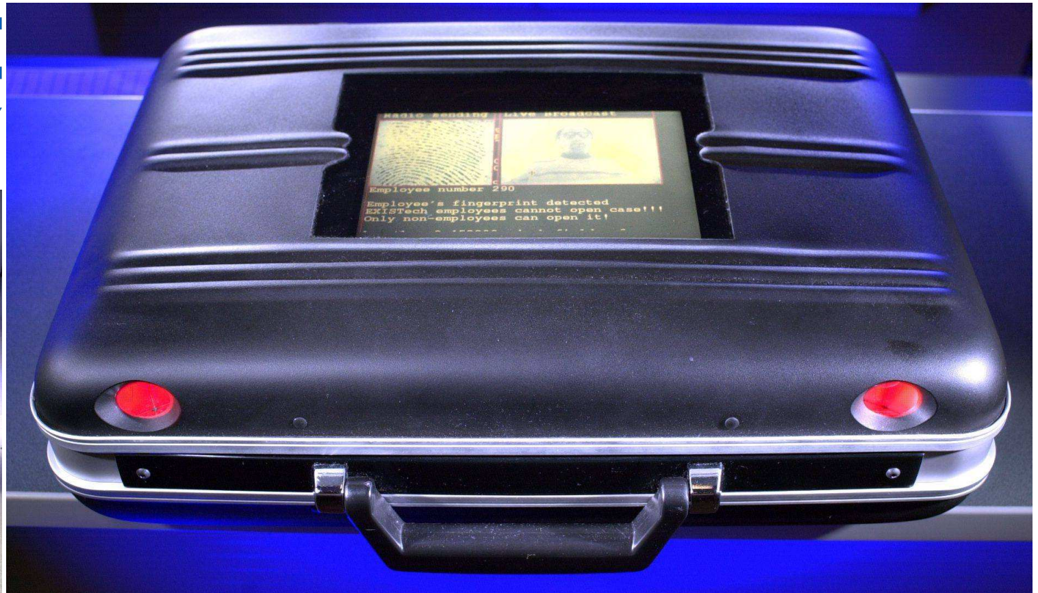
Fingerprint-scanning briefcase designed to be opened by anyone except the owner. Therefore, a security guard wishing to search the owner's case must submit to being fingerprinted! Leonardo Award for Excellence, S. Mann, 2004
