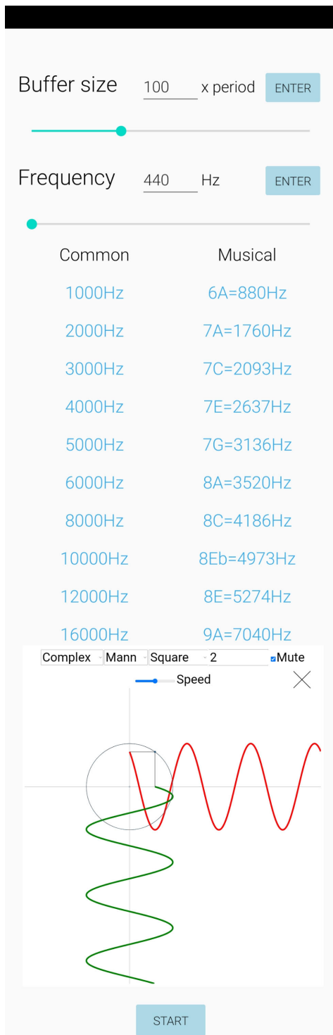
Figure 14. The SWIM simulator (SWIMulator™) app turns nearly any waterproof Android smartphone into a sonar and interactive XR (eXtended Reality) sonar teaching environment. The sonar can work in air, water, or even in sending sound waves through solid matter.
