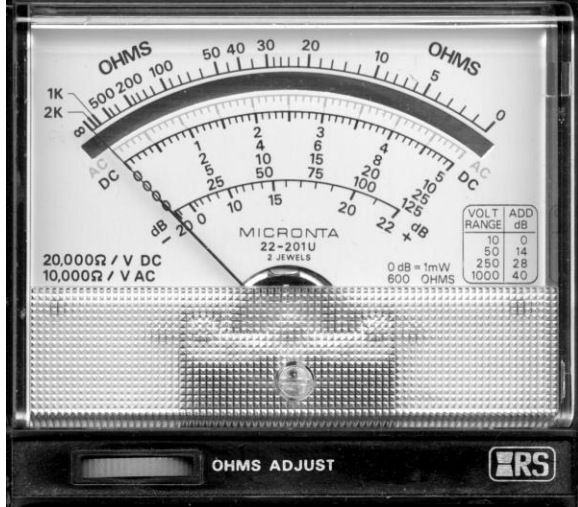
Figure 1: Typical resistance meter used in photocell experiment.
